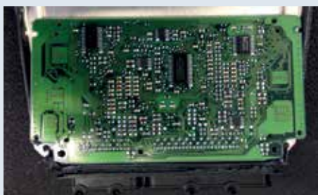
FIG. 4 THIS MEANS COMPLETELY REMOVING THE CIRCUIT BOARD FROM THE ECU CASING
