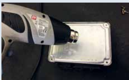
FIG. 2 THE ECU HAS TO BE WARMED UP TO BREAK THE SEAL. TOO MUCH OR NOT ENOUGH AND IRREVERSIBLE DAMAGE CAN OCCUR
