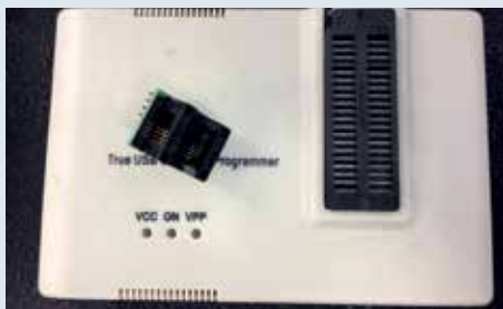
FIG. 7 ONCE THE MICRO IS REMOVED, IT HAS TO BE PLACED IN A SPECIFIC READING DEVICE WHICH IS ATTACHED TO A PC
