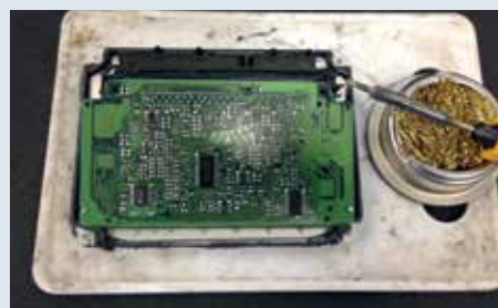
FIG. 6 THE DEVICE HAS TO BE REMOVED FROM THE CIRCUIT BOARD. THIS HAS TO BE EXECUTED PERFECTLY OTHERWISE PERMANENT DAMAGE MAY OCCUR
