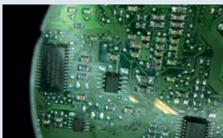
FIG. 5 CHECKING TO SEE THAT THE RIGHT MICRO DEVICE IS LOCATED. STRONG MAGNIFICATION IS REQUIRED FOR IDENTIFICATION
