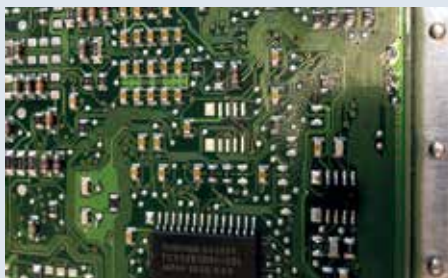
FIG. 11 THE ECU CIRCUIT BOARD HAS TO BE PREPARED TO ACCEPT THE FRESHLY MODIFIED MICRO
